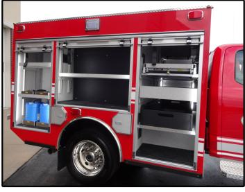
20 GPM @ 1,500 PSI Ultra High Pressure Fire Fighting System
