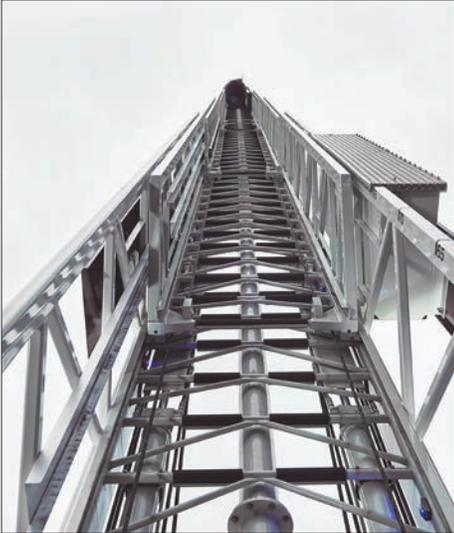
**AERIAL LADDER DESIGN:** All aerial ladder sections and primary load support members are designed with certified high-strength steel to ensure the highest quality with superior strength-to-weight ratios and minimal aerial ladder deflection.
