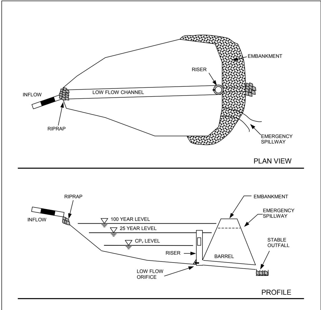
Figure 3.4.1-2 Schematic of Dry Extended Detention Basin
