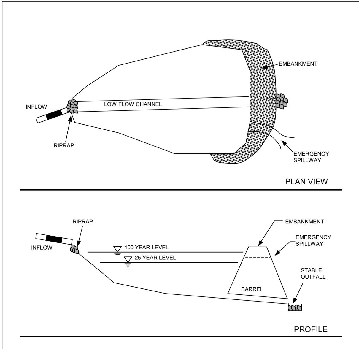
Figure 3.4.1-1 Schematic of Dry Detention Basin
