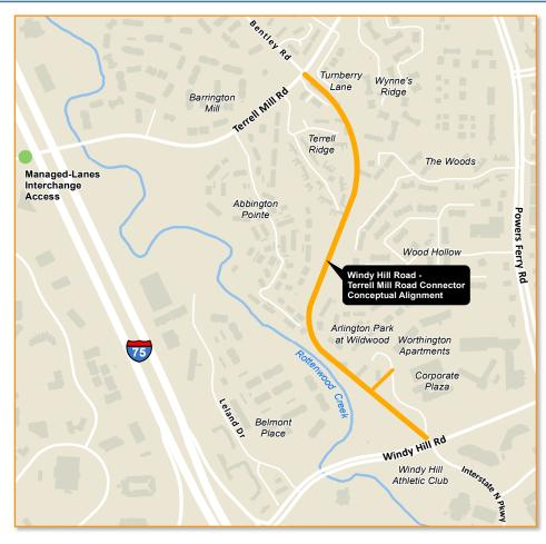
The Windy Hill Road - Terrell Mill Road Connector project is a proposed 0.80-mile limited-access, four-lane thoroughfare connecting Windy Hill Road to Terrell Mill Road. This road will begin at the existing intersection of Spectrum Circle/Interstate North Parkway and Windy Hill Road, and proceed north along a new location alignment to the existing intersection of Bentley Road and Terrell Mill Road.
