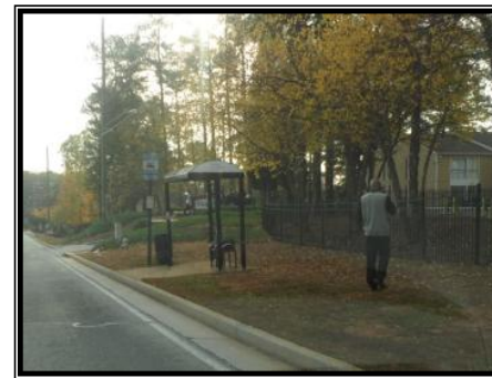
Six Flags Drive - Bus shelter with missing fiberglass siding and no sidewalks for approaching pedestrians.
