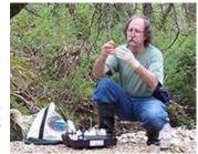
Chemical Monitoring is designed to teach volunteers about basic stream water chemistry and how to conduct the chemical tests using hand-held field equipment. The tests that volunteers are asked to conduct includes dissolved oxygen, conductivity, pH, and temperature.
