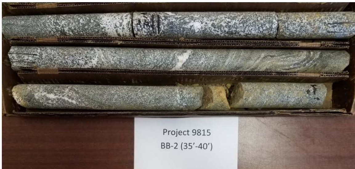
Photo 6: Boring BB-2 (35'-40') Recovery = 100%, RQD = 93%
