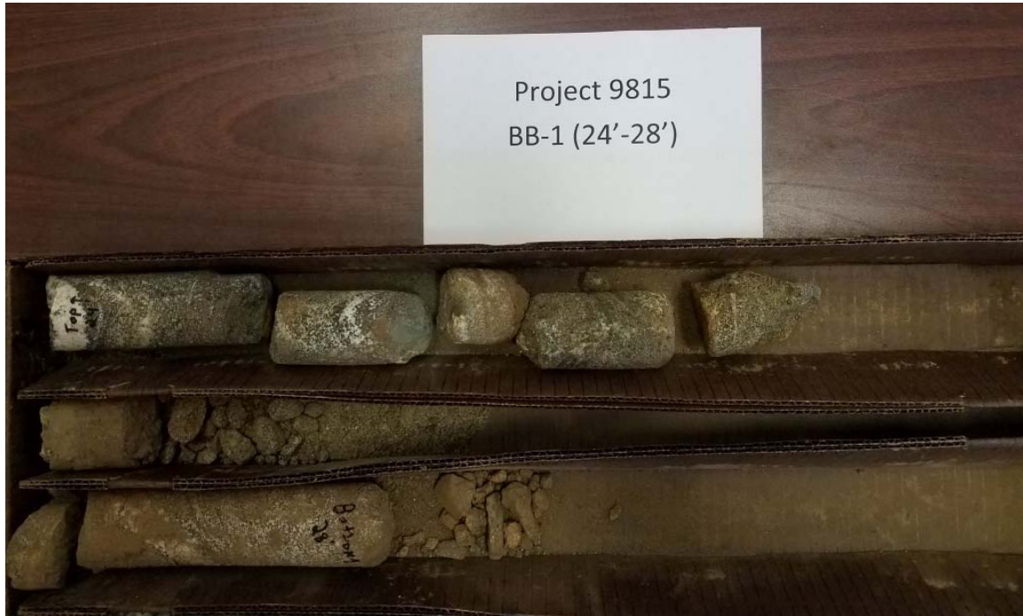
Photo 1: Boring BB-1 (24'-28') Recovery = 56%, RQD = 24%
