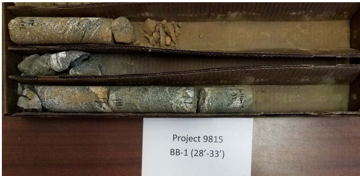
Photo 2: Boring BB-1 (28'-33') Recovery = 30%, RQD = 24%
