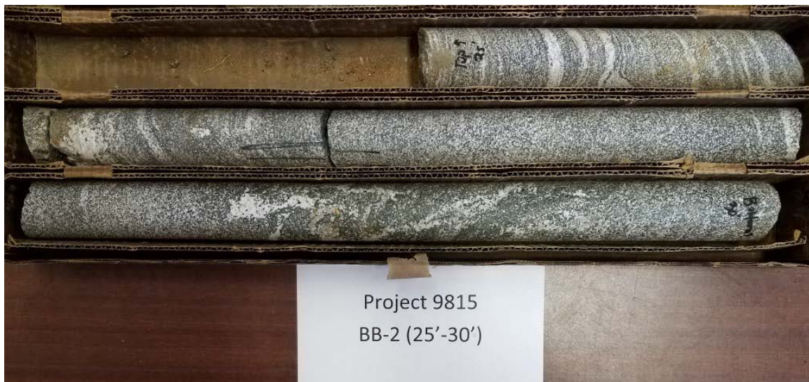
Photo 4: Boring BB-2 (25'-30') Recovery = 94%, RQD = 91%
