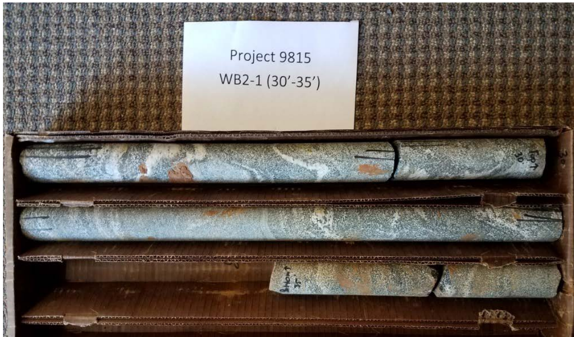
Photo 3: Boring WB2-1 (30'-35') Recovery = 98%, RQD = 98%
