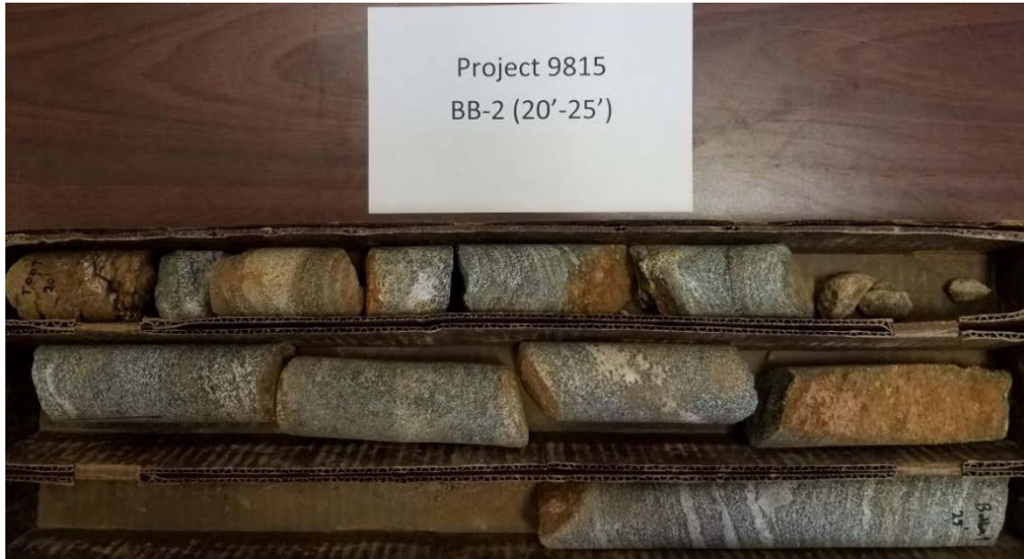
Photo 3: Boring BB-2 (20'-25') Recovery = 68%, RQD = 26%
