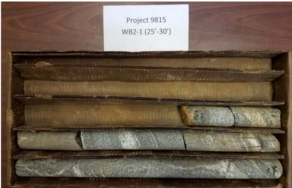
Photo 2: Boring WB2-1 (25'-30') Recovery = 92%, RQD = 87%
