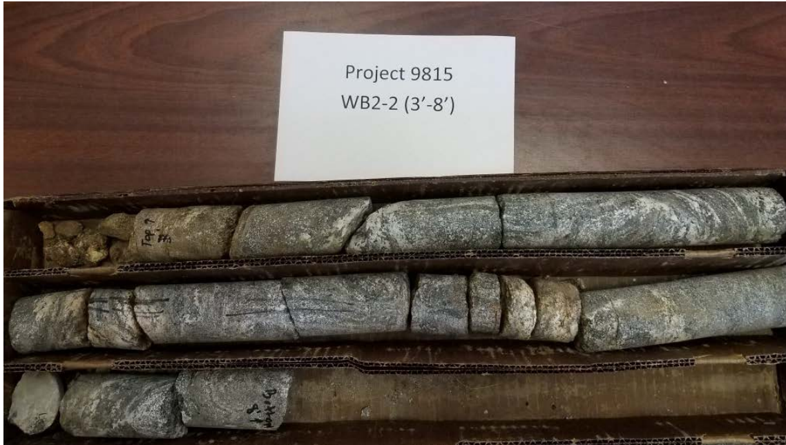
Photo 1: Boring WB2-2 (3'-8') Recovery = 87%, RQD = 43%
