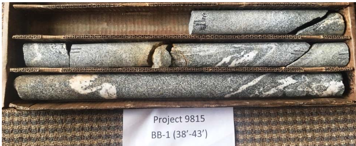
Photo 4: Boring BB-1 (38'-43') Recovery = 97%, RQD = 80%
