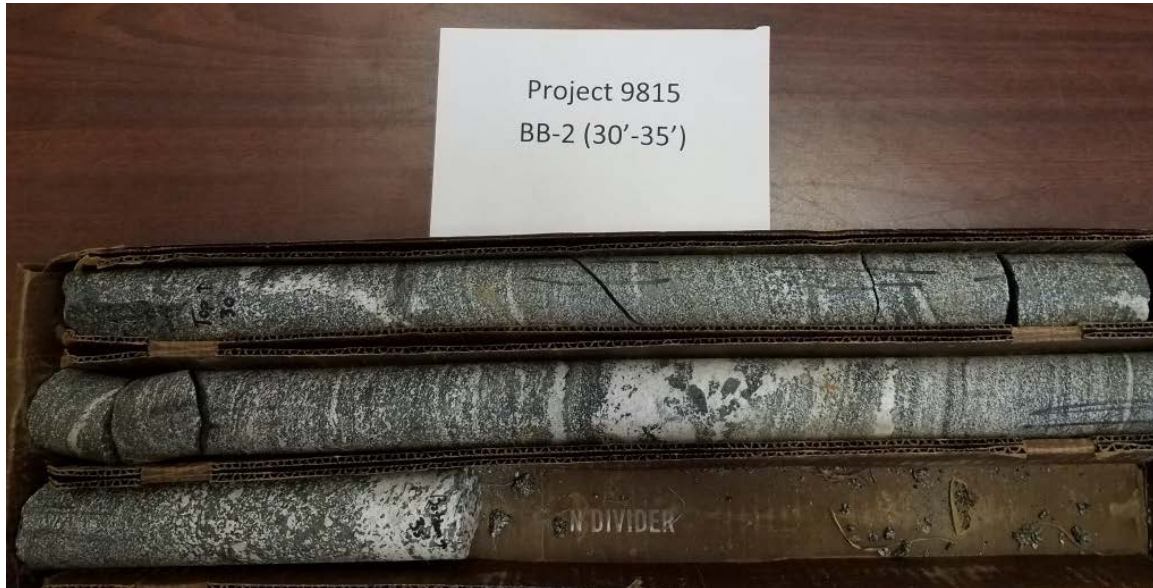
Photo 5: Boring BB-2 (30'-35') Recovery = 100%, RQD = 100%
