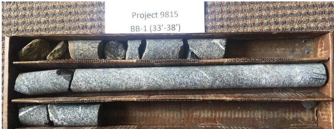
Photo 3: Boring BB-1 (33'-38') Recovery = 80%, RQD = 47%
