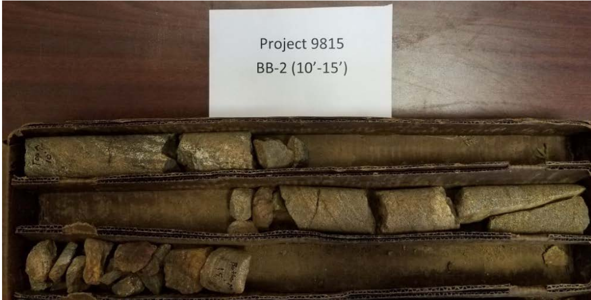
Photo 1: Boring BB-2 (10'-15') Recovery = 57%, RQD = 10%
