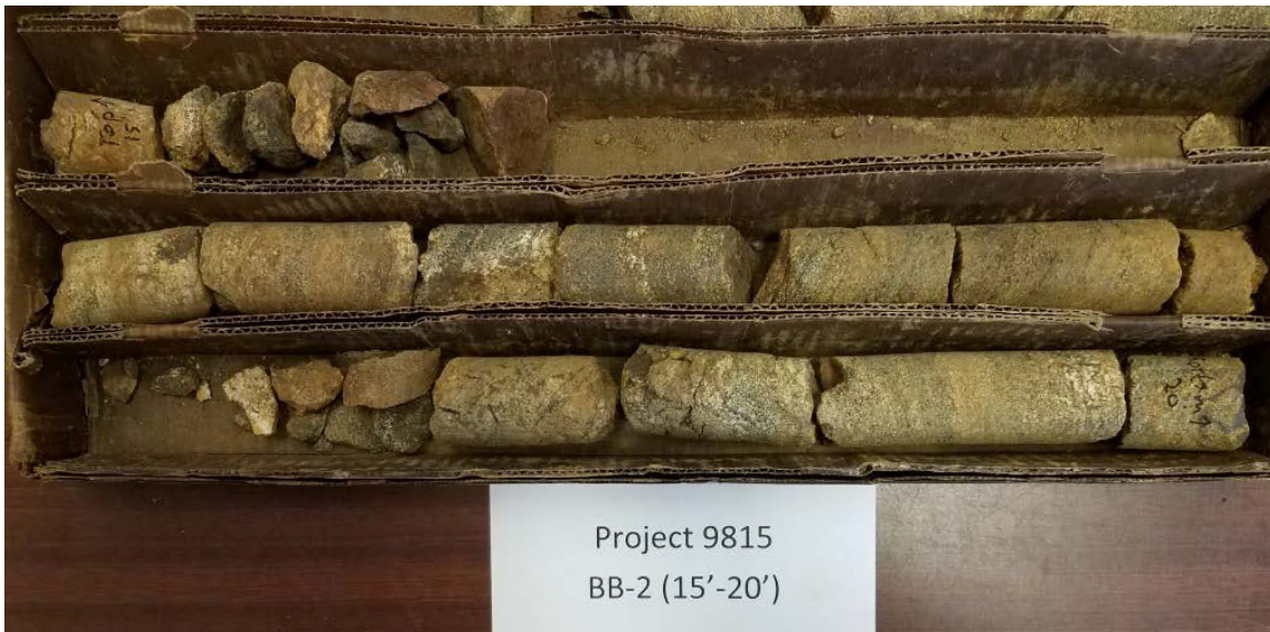
Photo 2: Boring BB-2 (15'-20') Recovery = 67%, RQD = 22%
