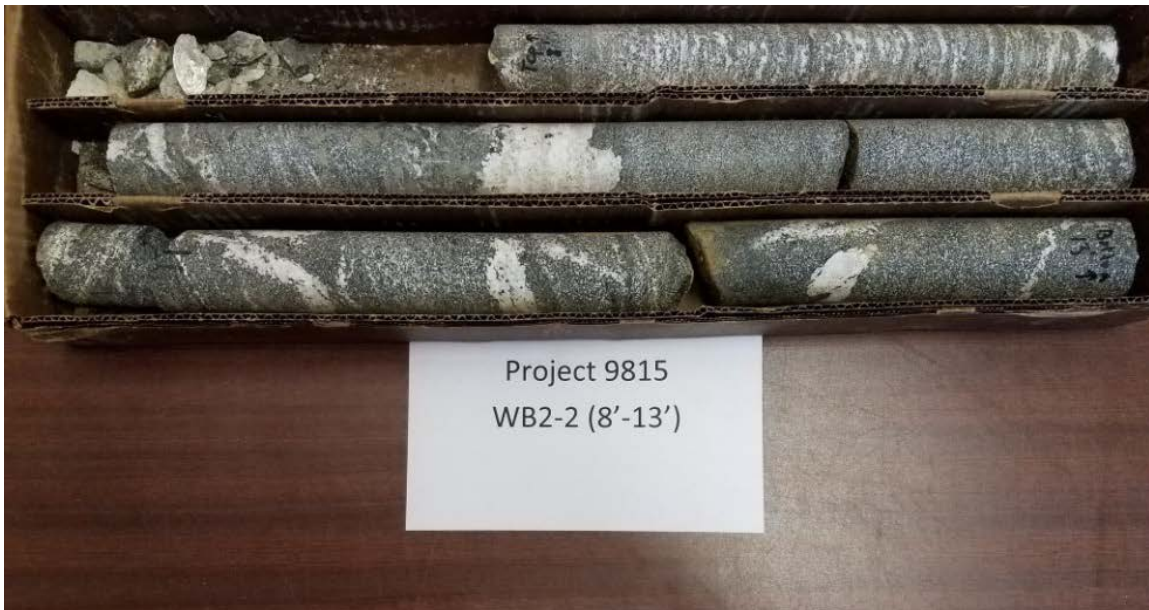
Photo 2: Boring WB2-2 (8'-13') Recovery = 97%, RQD = 97%
