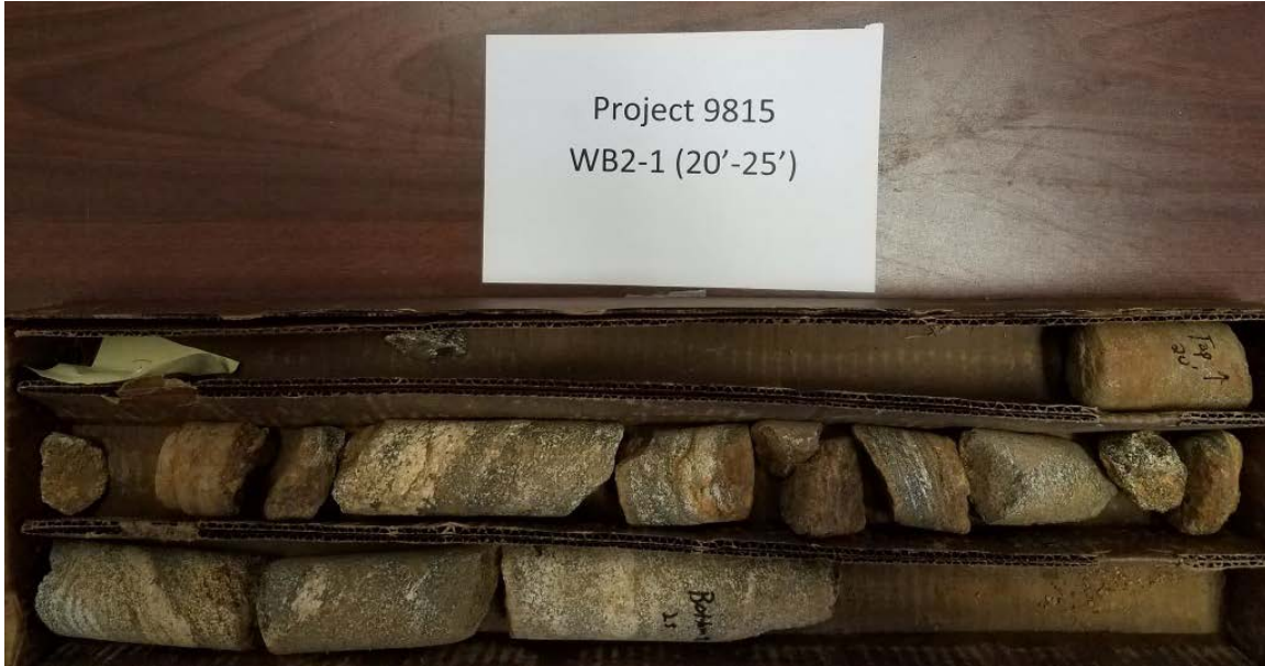
Photo 1: Boring WB2-1 (20'-25') Recovery = 63%, RQD = 29%
