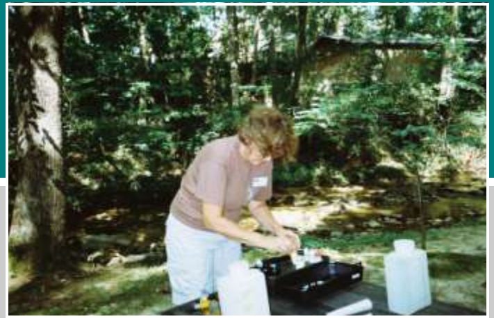
During our River Rendezvous, participants collect water samples and use the shallow water monitoring kit to determine pH, oxygen levels, conductivity, and temperature. They also collect water for additional evaluation including E. coli , turbidity, and solids.
