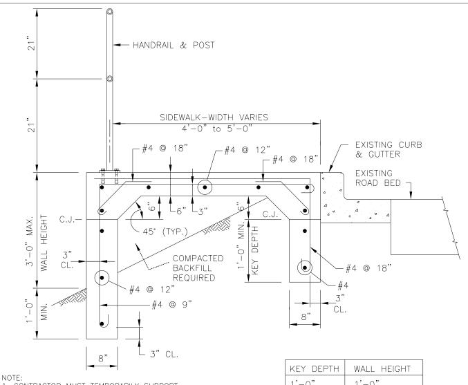
1. CONTRACTOR MUST TEMPORARILY SUPPORT FOOTING WALLS UNTIL TOP SLAB IS IN PLACE.
