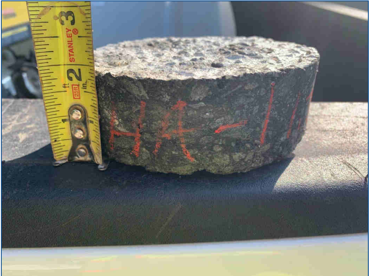
Photo 1 - HA-1 = Asphalt 1.75" Aggregate 8.5"
