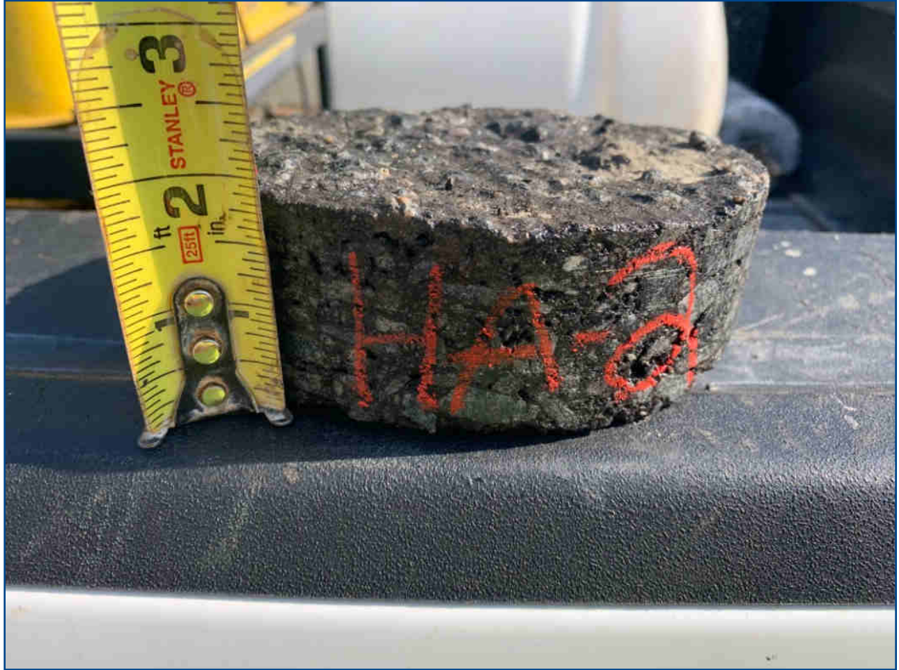
Photo 2 - HA-2 = Asphalt 1.75" Aggregate 8"
