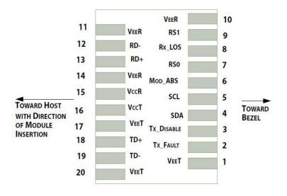
Pin-out of connector Block on Host board
