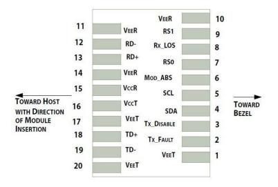
Pin-out of connector Block on Host board
