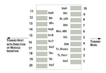
Pin-out of connector Block on Host board
