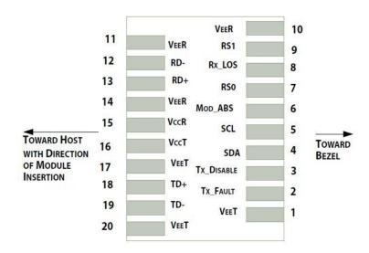
Pin-out of connector Block on Host board
