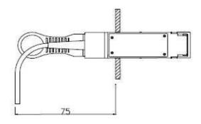
Clearance 75mm Is Required. Cable Type: Low Smoke Zero Halogen
