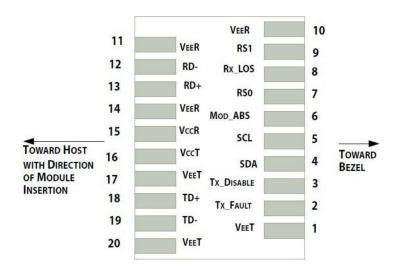
Pin-out of connector Block on Host board
