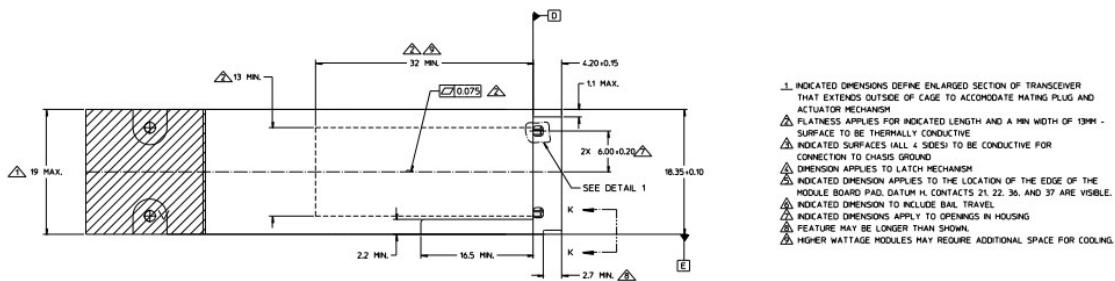
1. INDICATED DIMENSIONS DEFINE ENLARGED SECTION OF TRANSCIVER THAT EXTENDS OUTSIDE OF CAGE TO ACCOMMODATE MATING PLUG AND ACTUATOR MECHANISM.
