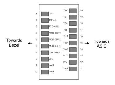
Pin-out of connector Block on Host board
