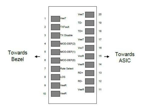
Pin-out of connector Block on Host board
