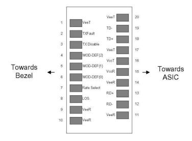
Pin-out of connector Block on Host board
