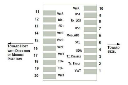
Pin-out of connector Block on Host board
