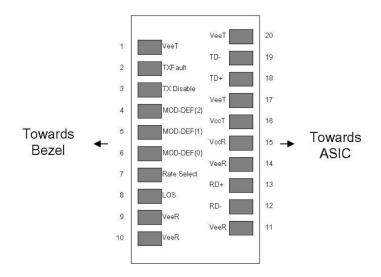
Pin-out of connector Block on Host board
