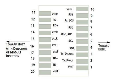
Pin-out of connector Block on Host board
