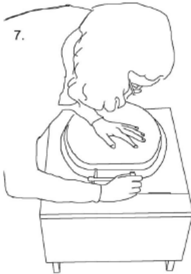
7. Mark holes for toilet seat attachment.
