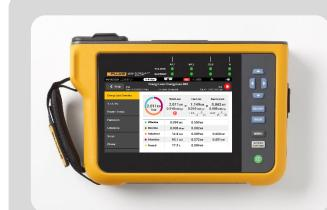
Measurement mode on Fluke 1775 and 1777 devices.
