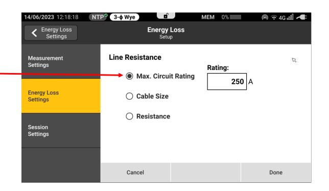
**Remember:** The Energy Loss Settings relate to the conductors connecting the load to the energy source.
