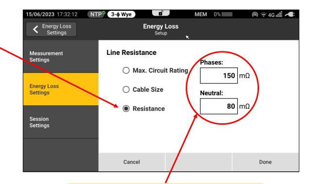
Please note: Values are in  $m\Omega$ . It is standard practice for the neutral conductor to be 2x the size of the phase conductor to minimize losses.
