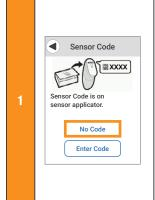
When setting up the receiver or inserting a new sensor without using a sensor code, on the Sensor Code screen, tap **No Code**.
