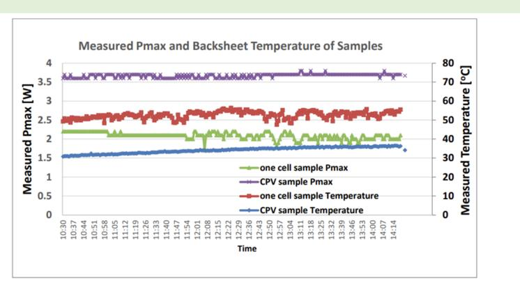
Blue plot/right axis = temperature of cell in module Red plot/right axis = temperature of control cell
