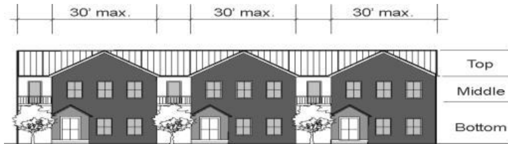
Figure 41. Multifamily facade articulation example. Note roofline changes, use of balconies, and delineation of the facade’s top, middle, and bottom. Changes in materials or siding (noted by use of different shades here) can also be effective in breaking up the scale of the building and adding visual interest.
