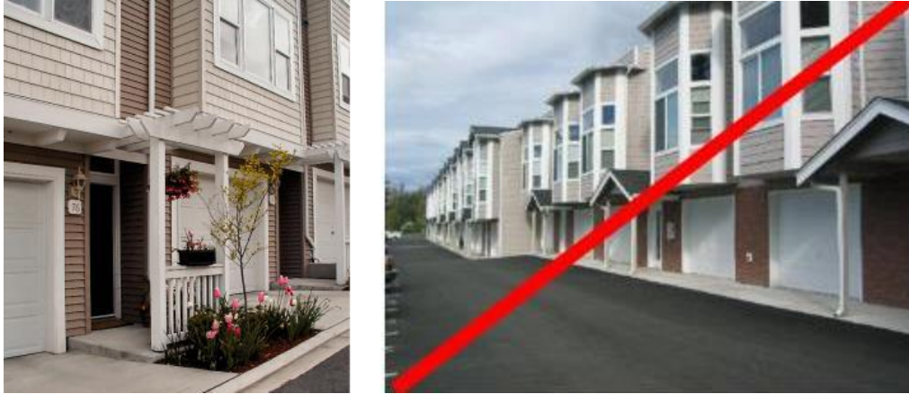
Figure 15. Acceptable (top) and unacceptable (bottom) townhouse parking garage entrance examples.
