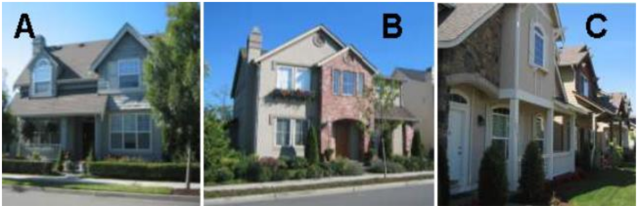
Figure 6. Examples of how houses can meet architectural detail criteria. Image A includes decorative windows, building material treatment, and roofline elements. Image B includes decorative brick use, window treatments, entry design, and ventilation circles. Image C includes decorative building materials, door/entry feature, windows, and roofline elements.
