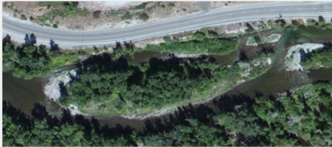
Figure 3: GUT Tier 1 output for CHaMP reach (ENT00001-1BC1) on the Entiat River (WA). This site is a low gradient (0.5%), partly confined, multi-threaded reach with an average bankfull width of 18 m. Data was collected in 2014 using total stations
