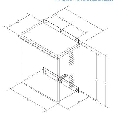
NOTE: ENCLOSURES ARE SUPPLED WITH (6) KEYHOLES SIZED FOR A MAXIMUM 5/16 (0.313") MOUNTING BOLT (B-1) AND 3/8 (0.375") MOUNTING BOLT (B-2).
