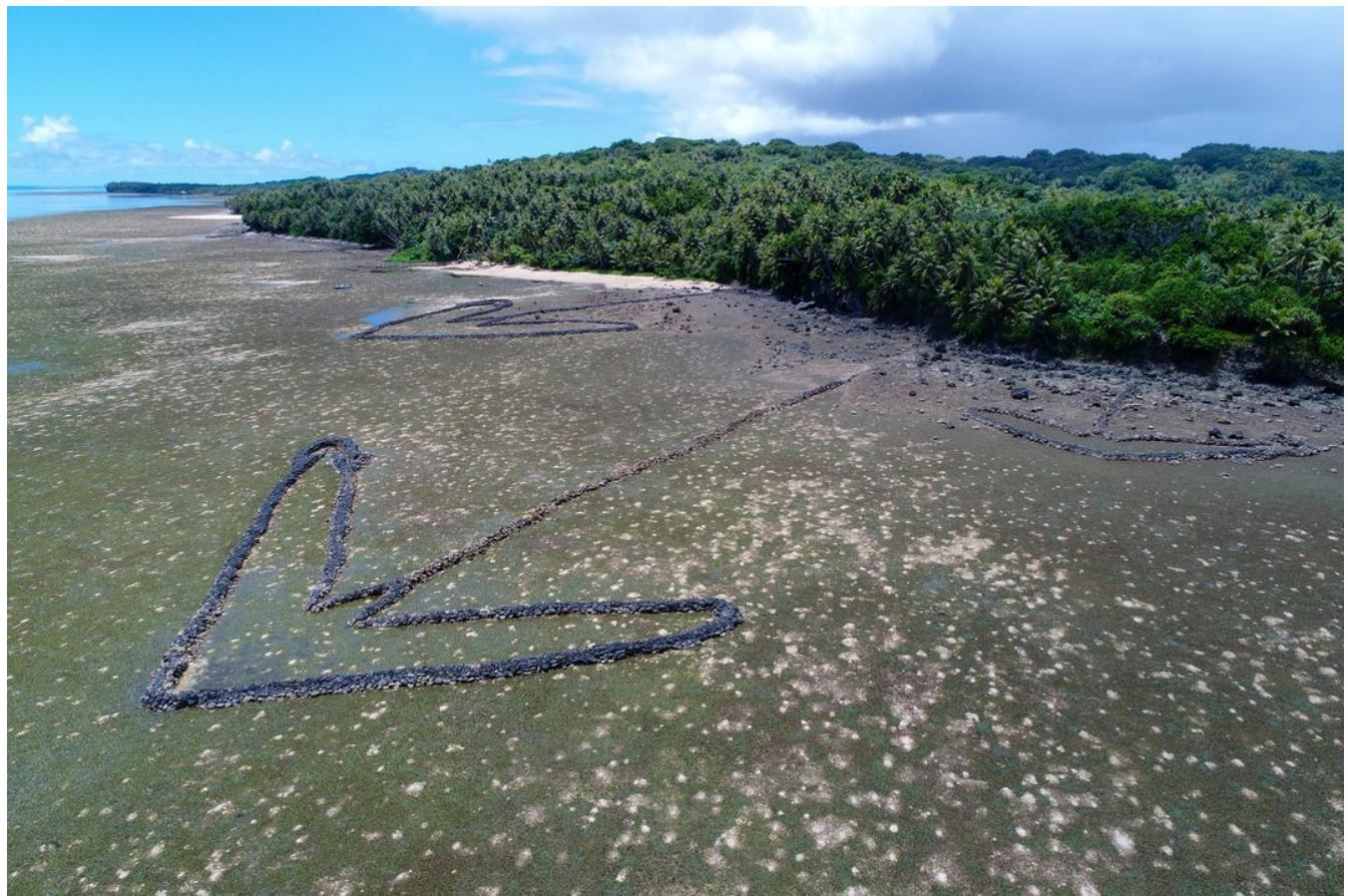
Stone tidal fish traps point toward the sea on the islands of Yap in the Federated States of Micronesia. These structures lie underwater at high tide and catch fish as tides drop. They have been used for more than 1,000 years ago. Photo by Bill Hatcher
