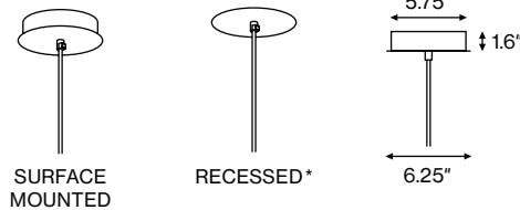
\*For recessed canopy, cut 6" dia hole and recess j-box or mounting structure by 1.5"
