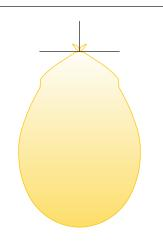
78° WIDE FLOOD LUMINOUS FLUX: 2373LM **INPUT POWER: 25W** SPACING CRITERION: 1.08
