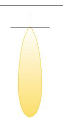
30° NARROW FLOOD LUMINOUS FLUX: 2678LM **INPUT POWER: 25W** SPACING CRITERION: 0.50
