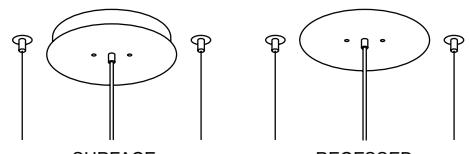
For recessed canopy, cut 11" dia hole and recess j-box or mounting structure by 1.5"
