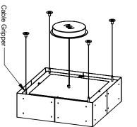
A Attach canopy to junction box with (2) mounting screws (not included). Use curved slots in canopy.
