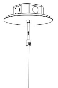
Lift the strain relief upward and screw it into the canopy. Tighten strain relief set screw once strain relief is in place.
