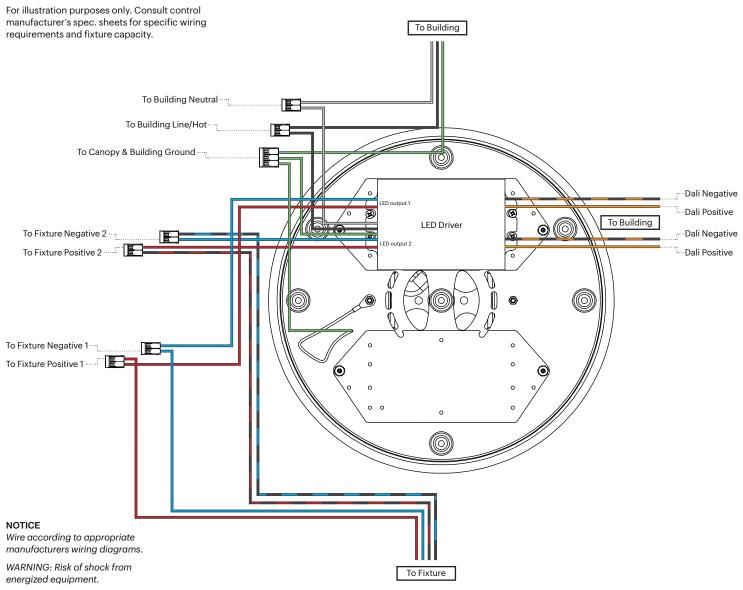
Always turn power OFF and lock out during fixture installation.
