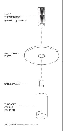
Thread the adapter onto the all thread until firmly secured against ceiling as shown.
