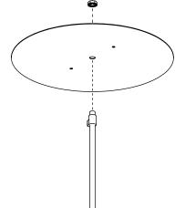
(5) Lift the dress plate upward and align the decorative nuts with the standoffs protruding from the canopy.
