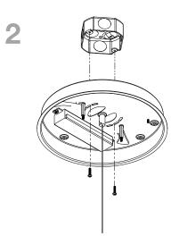
Push the connections and all excess wires into junction box.
