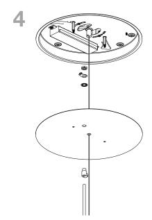
Pass enough length of the power cord through Strain Relief and secure strain relief onto the dress plate using washer, ground lug and nut
