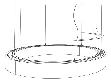
Locate the LED lid labeled with a number 1 on the underside. This is the first lid to be installed and will have a silver power cord located on one end. The first lid should be possitioned on the fixture so that the silver power cord is directly beneath one of the ceiling canopies.
