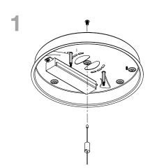
Pull S.S cable through coupler and thread coupler onto 1/4-20 Button head cap screw at center hole until coupler is firmly secured against the underside of the canopy
