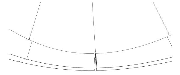
Only after the first shade section is leveled and at the appropriate height, proceed to the next shade section. Raise the second shade section into place and attach the (2) corresponding s.s. cables. Only after the (2) s.s. cables have been attached should you attempt to attach the first two shade sections to one another.
