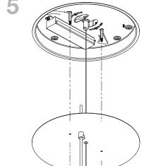
With canopy secured to junction box and Strain secured to dress plate, pass S.S cable through center hole in canopy. Then slide the dress plate up the cable and secure dress plate using decorative cap as shown
