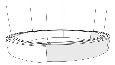
Proceed with the next shade section in the same manor as described previously, making sure to level each section and secure the fasteners between each shade until the entire ring is assembled. Proceed with the installation of the LED lighting and lids on the following page.
