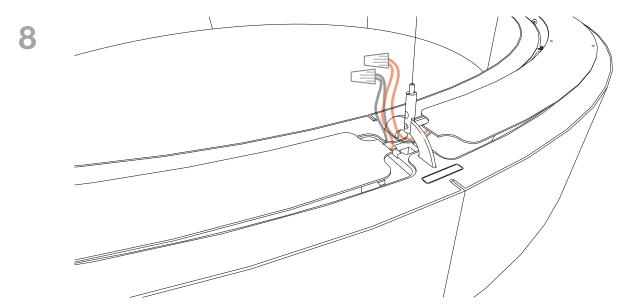
Locate the next LED lid with a number 2 on the underside. Feed the positive and negative leads from the second lid under the hanger and connect them to the corrisponding leads on the first lid with the provided connectors.
