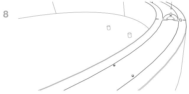
Install (2) nickle plated decorative caps to secure each lid to the top diffuser. The final step in the installation process is to wire the silver power cords from the fixture to the canopies above. Please refer to the wiring diagram on page XX-XX for additional information and wiring instructions.
