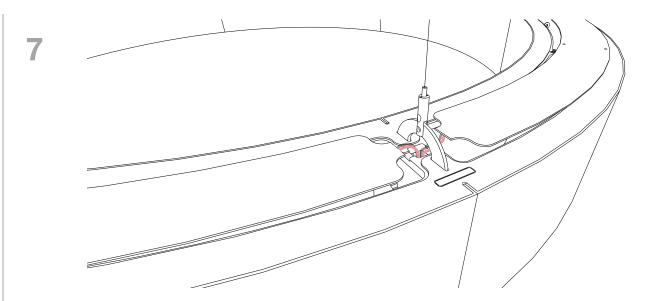
Gently tuck the connectors into the compartment under the hanger, until the lids lay flat on the top of the fixture. Proceed in this same manor until all lids are installed on ring.
