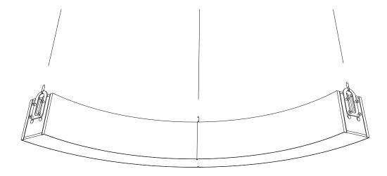
Locate the "CORNERSTONE" shade section, which has support hangers factory installed on both ends. Raise the cornerstone section to the desired height and attach the (3) cables by feeding the free end into the cable grippers. Before proceeding to the next shade make sure the shade section is at the proper height and is level. WARNING depending upon size it can be very challenging to adjust the height and level the fixture once all the shade sections are suspended.
