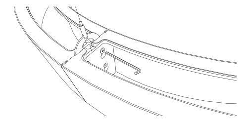
Check second shade for level, the seam between the top and bottom diffusers of both shades should be aligned. Tighten the fasteners between shades with the provided allen key.
