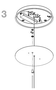
Pass enough length of the power cord through Strain Relief and secure strain relief onto the dress plate using washer, ground lug and nut
