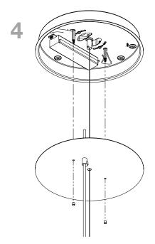
With canopy secured to junction box and Strain secured to dress plate, pass S.S cable through center hole in canopy. Then slide the dress plate up the cable and secure dress plate using decorative cap as shown
