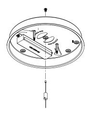
Pull S.S cable through coupler and thread coupler onto 1/4-20 Button head cap screw at center hole until coupler is firmly secured against the underside of the canopy
