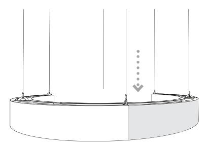
With the hardware from shade 1 engaged in to the keyway slot in shade 2 shown in gray lower the end of shade 2 to connect the shade sections.
