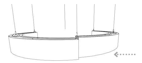
Attach the second shade section to the first shade section by lifting the end of the shade slightly until the hardware engages the keyway slops on shade section 2 shown in gray.
