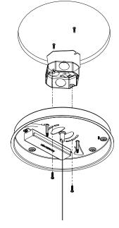
Secure junction box onto the cover plate with fasteners. Push the connections and all excess wires into junction box. Secure canopy to junction box with screws.
