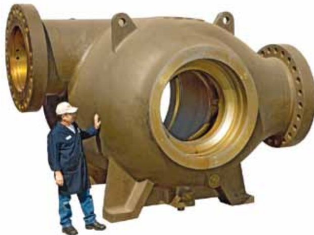
C85 Gas Compressor
