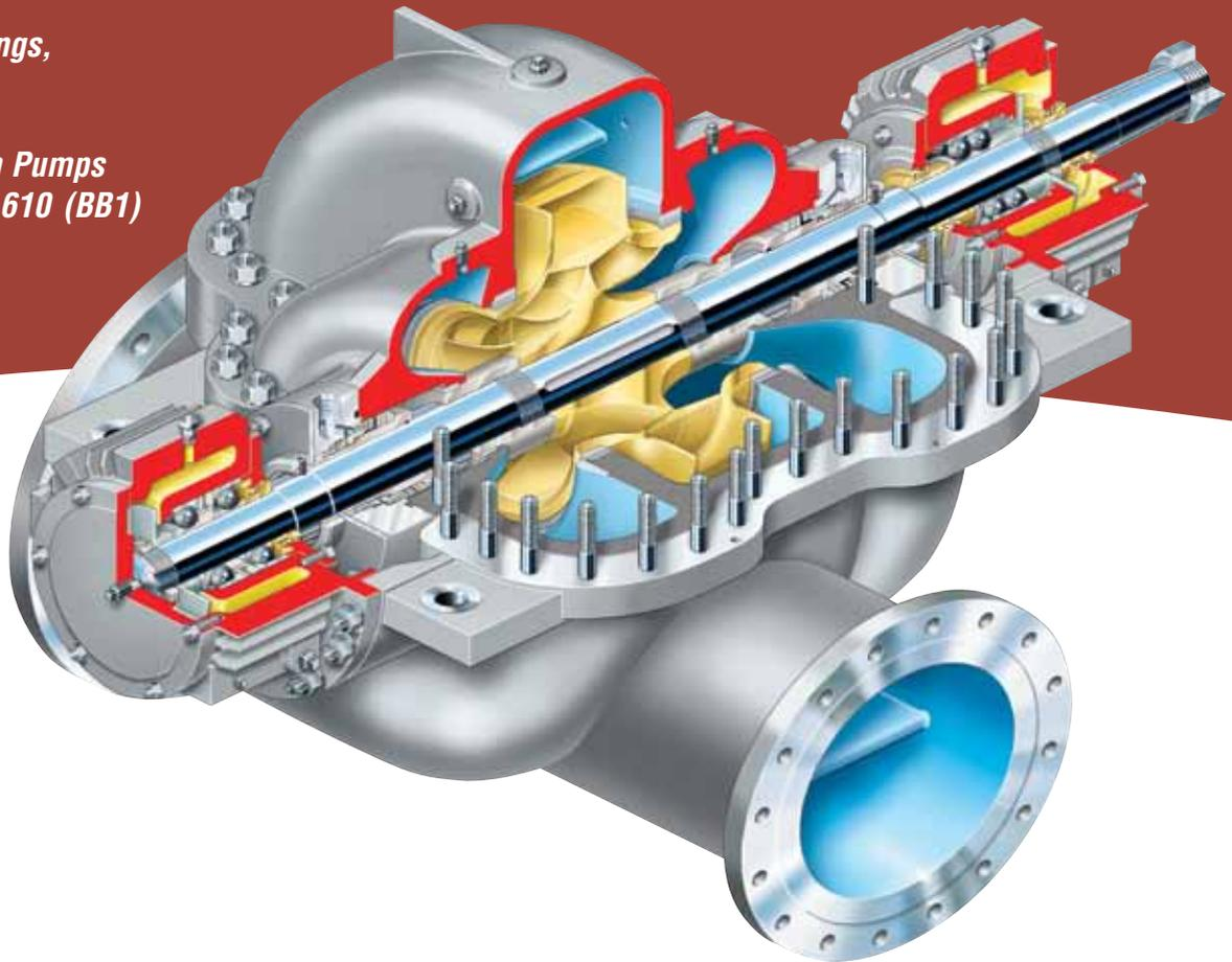
*The Flowserve LPN is an axially split, single-stage pump designed to ISO 13709/API 610 (BB1), latest edition. With a double-suction impeller, the LPN is a natural solution for many low NPSH applications, such as those found in water and hydrocarbon transfer service.*
