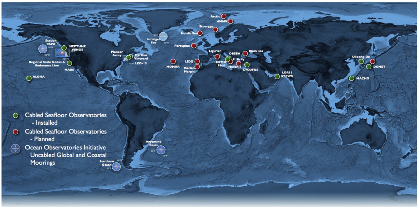
Fig. 4. Locations of installed (green dots) and planned cabled seafloor observatories (red dots). Many of the sites located around the perimeter of Europe are part of the extensive ESONET (European Sea Floor Observatory Network) array planned to include 5000 km of submarine fiber optic cables ( http://www.oceanlab.abdn.ac.uk/research/esonet.php ). Also shown are the locations of high latitude uncabled mooring arrays (Papa, Irminger, Southern Ocean, Argentine basin), the coastal arrays (Pioneer, Washington and Endurance Lines) that are components of the NSF's Ocean Observatories Initiative.
