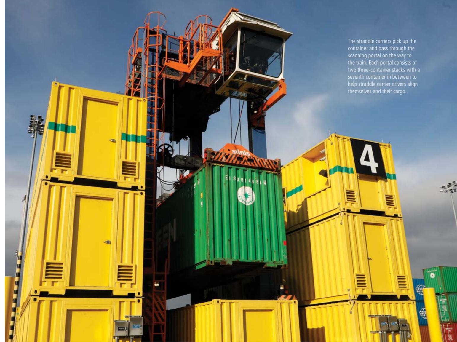
The straddle carriers pick up the container and pass through the scanning portal on the way to the train. Each portal consists of two three-container stacks with a seventh container in between to help straddle carrier drivers align themselves and their cargo.
