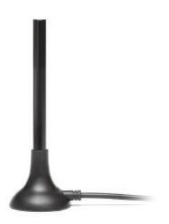
The Lyra Antenna is a small, high-performing antenna that comes standard with OptConnect mylo. With a magnetic mount that can be used on any ferromagnetic (iron or steel) metal surfaces, it is ideal for ATMs, POS, sensor applications, and more. The Lyra Antenna delivers stable omni-directional gain and efficiencies across all common 4G/5G, cellular bands.
