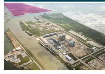
Federal seismic requirements for Puget Sound Energy's tank design and construction are more rigorous than for bridges and overpasses. Construction of the facility is required to exceed the standard to withstand an earthquake expected every 2,450 years with no loss of LNG, compared to bridges and overpasses that are built to withstand 1,000-year earthquakes.
