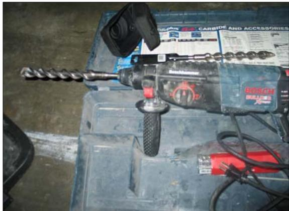
Roto-hammer used to Obtain Concrete Wall Samples
