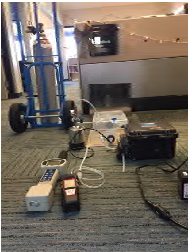
Photo 19: Typical sub-slab soil gas sample set up
