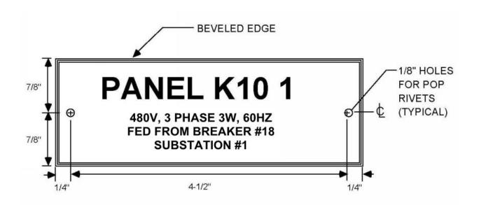
NOTE: LETTERING ON FIRST LINE IS 3/8" HIGH. ALL OTHER LINES OF LETTERING ARE 1/8" HIGH WITH 1/8" SPACING BETWEEN LINES.
