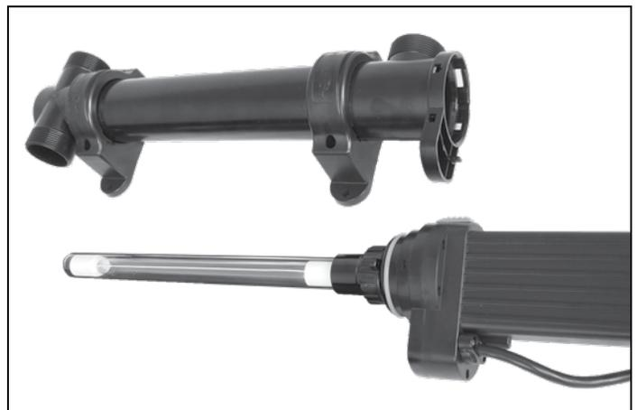
5. If replacing or removing the quartz sleeve remove the threaded plastic collar at the base of the quartz sleeve and remove the quartz sleeve.
