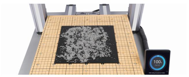
2. Clean the finished work and the machine with a dust collector, and then remove the finished work using the diagonal pliers.
