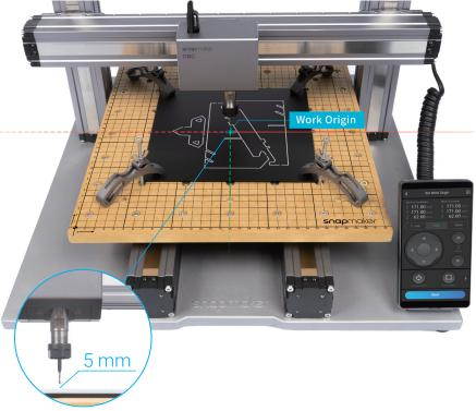
3. Place the Calibration Card or a piece of A4 paper between the CNC Bit and the material. Keep adjusting the height of the CNC Bit using **Z-** or **Z+** buttons until you feel slight resistance when you pull out the Calibration Card, and it should be wrinkled when you push it forward. Tap **Set Work Origin**.
