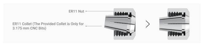
2. Put on the CNC Safety Goggles. Insert the CNC Bit into the ER11 collet (Flat End Mill is required for our provided model). Keep pushing the CNC Bit until its end bottoms against the shell of the ER11 collet.
