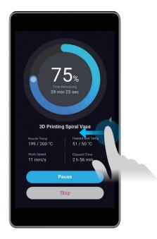
If poor adhesion occurs, swipe left on the printing progress screen and try adjusting the Z Offset. Or you can try leveling the Heated Bed again by selecting **Calibration**. Make sure the tip of the nozzle is clean before you calibrate the bed.
