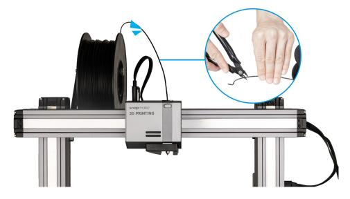
2. Tap **Start** on the **Load Filament** screen. After the temperature reaches the target temperature, tap **Load** and then gently push the filament into the 3D printing module until you can feel the motor pulling the filament in.
